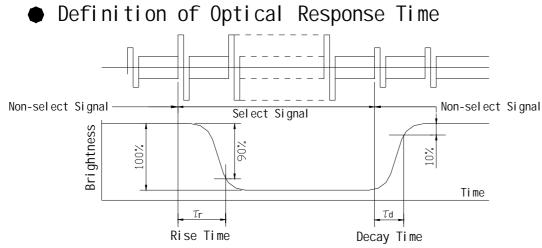
In case of Negative type, wave from of changing brightness becomes reverse (Non Select Signals: 0%, Select Signals: 100%
